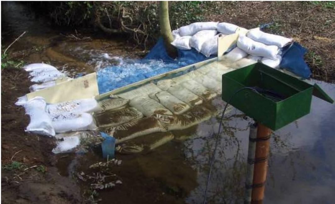
Gauging structure for automated logging of stream flow
