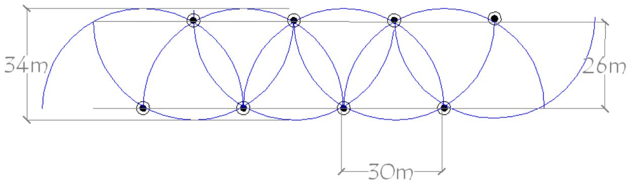
With this type of system the sprinkler spacing can be up to 30m, triangular and head-to-head. Such a system affords a considerable reduction in cost (relative to the 20m full-circle system) due to;
