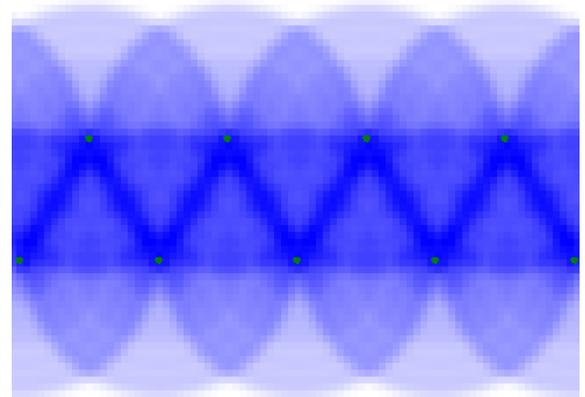
There is some scope here to introduce a more cost-effective solution that involves irrigating only the fairway and not the rough. This is only really possible if the fairway width is  $\leq 30\text{m}$ . For such circumstances a twin-row, long-radius, part-circle, system is possible.
