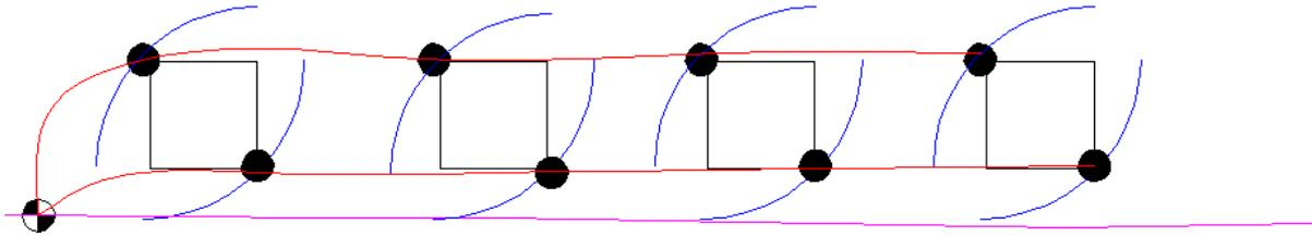
The previously illustrated conventional tee system has 3 tees (10m x 10m, 20m x 10m and 10m x 10m), the “value-engineered” system above has four tees (each 10m x 10m) so the total area of teeing surface is identical (400m<sup>2</sup>). So despite having more tees (4 v. 3), the value engineered system will have a less costly irrigation system because
