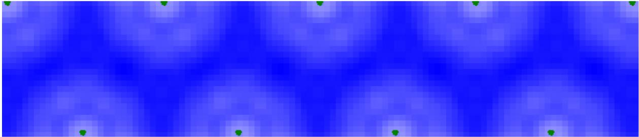
The downside is that the rough does not get irrigated, although it is possible to increase the arcs of the sprinklers up to 220°. Any greater than 220° and there is excessive overthrow.
