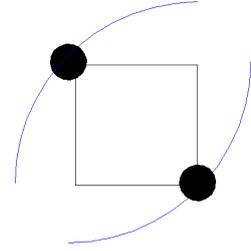
Small rectangles are undesirable as they require 3 sprinklers and result in more wasted water if the arcs are matched at  $180^\circ$ .
