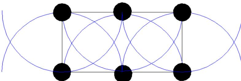
However this results in “wasted” sprinkler coverage to the front and back of the tee; this may or may not be desirable depending on the type of golf course and its environment.
