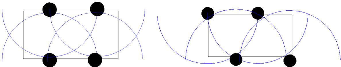
Furthermore the rectangular tee with 6 sprinklers has the problem of un-matched precipitation; there are 4 sprinklers with 90° arcs and two sprinklers with 180° arcs. For the same sprinkler/nozzle, the precipitation rate is twice near the corners of the tee as it is in the middle of the tee, resulting in a dry spot in the middle of tee (see right). The dry spot can be avoided if the 90° and 180° sprinklers are operated by separate valves – which adds yet more cost.
