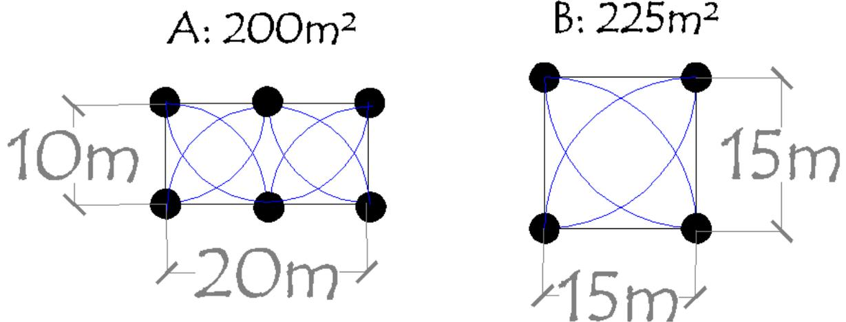
Tee A is smaller than tee B but requires 50% more sprinklers. To irrigate a rectangular tee with merely 4 sprinklers results in either poor uniformity of application or overthrow.
