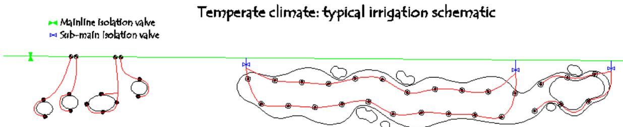
By fitting the sprinklers directly on the mainline you can reduce the amount of pipe and cable that has to be installed. However this should be done with caution and safeguards implemented to ensure continuity of downstream flow. The example below shows multiple isolation valves to enable the individual isolation of each main pipe so that in the event of a problem downstream flow can be maintained in the other pipe.
